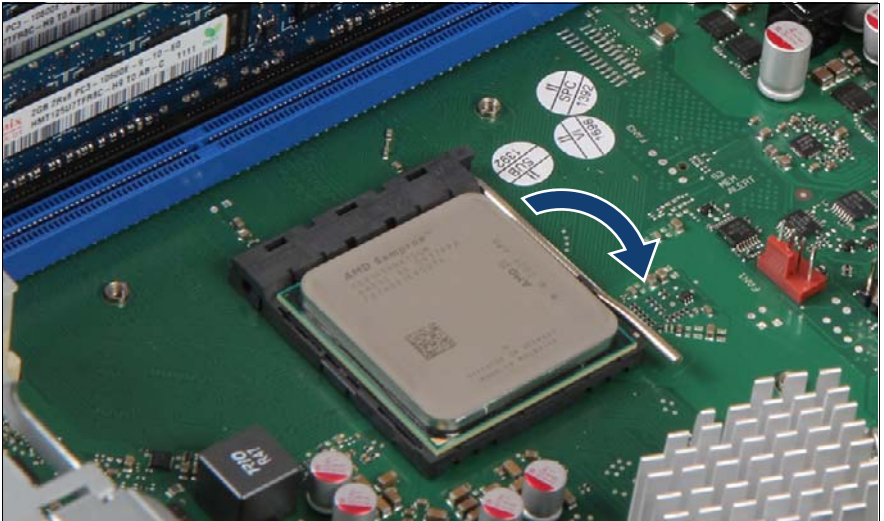
Figure 122: Latching the socket lever
